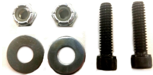
(2) 1/4-20 x 1 SHCS, washers and nylock nuts
